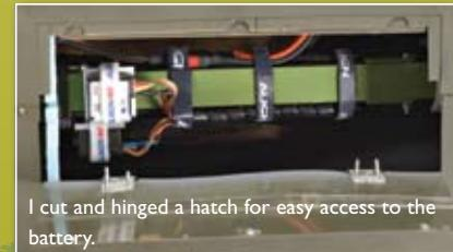
I cut and hinged a hatch for easy access to the battery.
